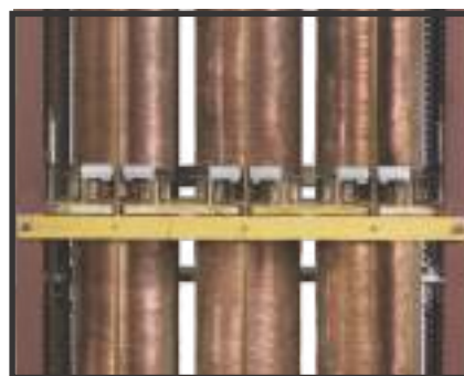
Inner view of Regulator with Carbon Roller Assembly
